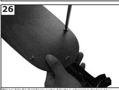
Place blade holders onto blades aligning holes in blade holder with holes in blade. Make sure that the side of the blade you select is facing downward. Install 3 screws and fiber washers to back side of blade as shown. Tighten screws securely. Repeat this process 4 more times until all blades are assembled.
